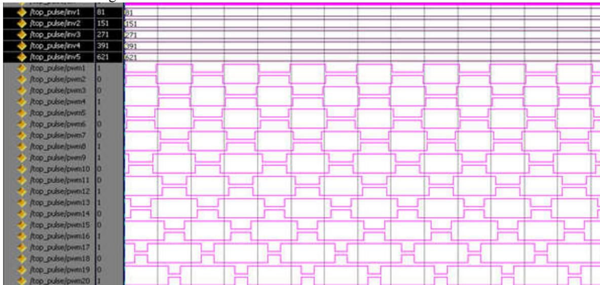
**Figure.9 Gating pulse output from Modelsim for the 20 switches of MLI with MI as 0.8**
