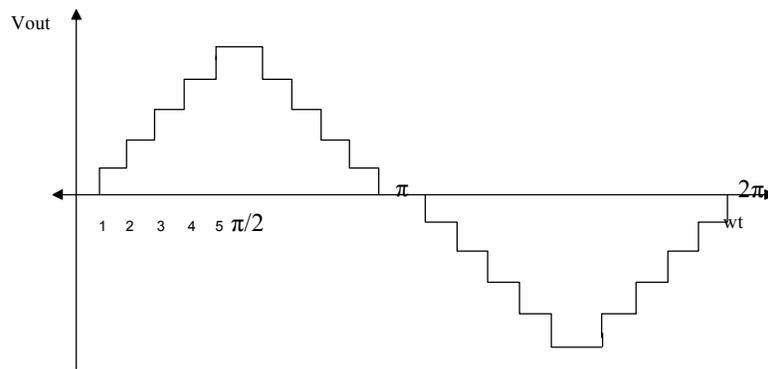
Figure.2 Output voltage waveform of 11-level cascaded MLI
