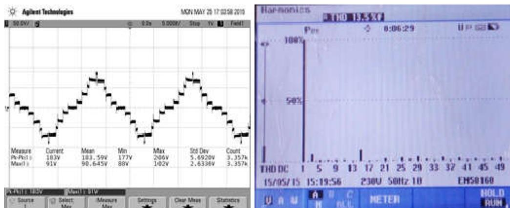
Figure.12 Inverter output voltage & harmonic spectrum for MI = 0.7
