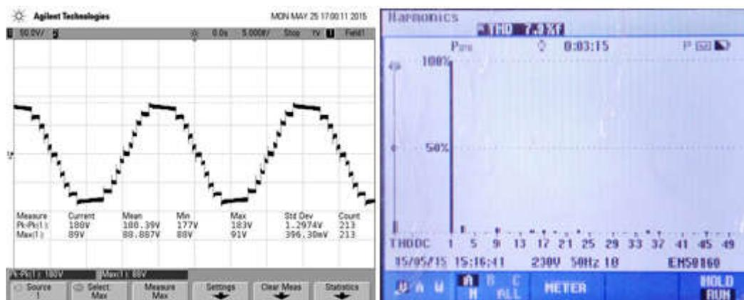
Figure.11 Inverter output voltage & harmonic spectrum for MI = 0.8
