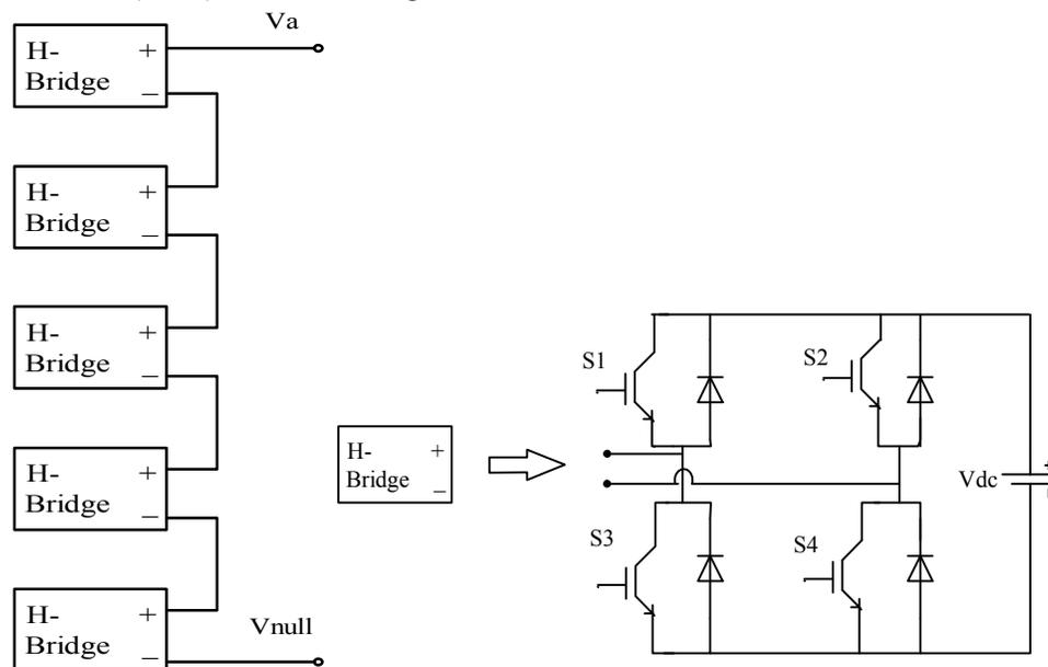
Figure. 1 Structure of eleven level cascaded H bridge MLI
