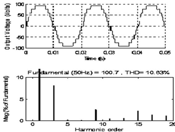
**Figure.3 Eleven level stepped waveform and Harmonic Spectrum of MLI with 0.8 as MI**
