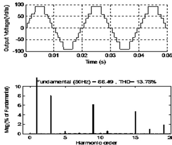
**Figure.4 Eleven level stepped waveform and Harmonic Spectrum of MLI with 0.7 as MI**
