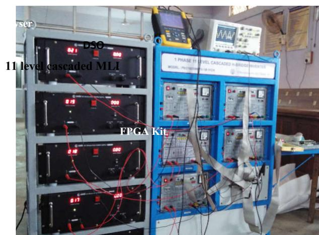
**Figure.10 Experimental Setup of Eleven Level Cascaded MLI**
