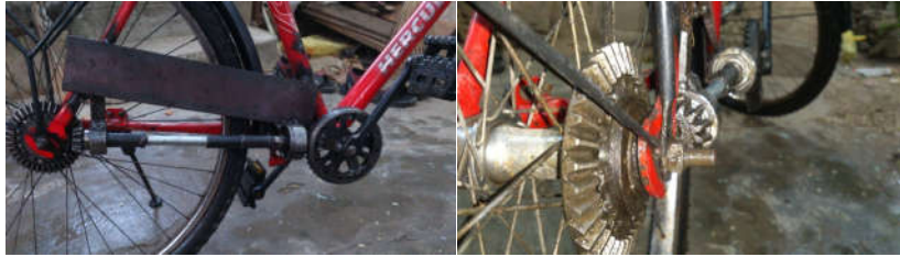
Figure13: Actual View of Power Transmitting Mechanism
