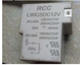
Figure4.1 Relay RCC L90CSDC12V
