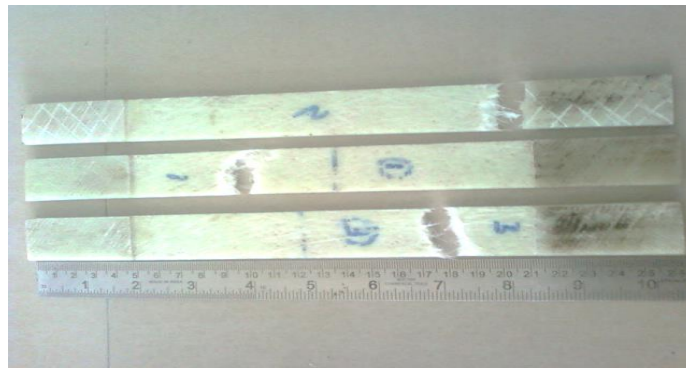
Figure.3: E-glass Chopped Strand mat/ Epoxy specimen after the Tensile Test
